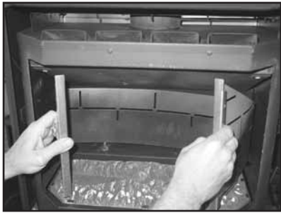
Figure 8.4 Holding both sides of the metal refractory brick piece, pull slightly together and rotate out of the firebox.
